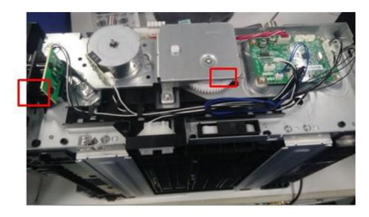
**Step2**: Confirm that plug wire into the appropriate side as shown above picture. If the status is NG, you can confirm it after starting printer. If the status is ok, but still have troubles with printer, it may cause by motor or board.
