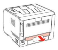
**Step2**: Remove the jammed paper from the duplex unit.
