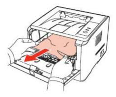
**Step4:** After removing the jammed paper, reload the toner cartridge and close the front cover, then the printer will automatically resume printing.
