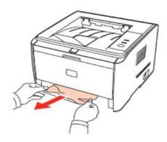
**Step3:** After removing the jammed paper, reload the tray into the printer, and restore the printing by pressing the button on the panel.
