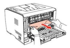
**Step4:** Remove the jammed paper and close the fuser door and the rear cover, then the printer will automatically resume printing.
