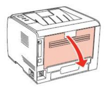
Step2: Open the fuser door using the handles on both sides.
