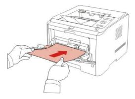
When you put paper into the multifunctional input tray, this printer will select the printing paper inside multifunctional input tray in priority.
