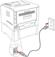
Note: • Before installation or moving of the optional tray, please cut off the power supply to the printer.
