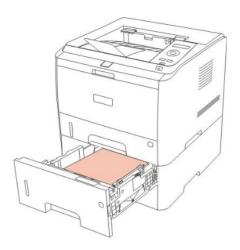
Note: The optional tray supports automatic duplex printing of common paper only. Do not put any special printing medium into the option tray.
