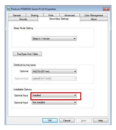
d) When the multifunctional input tray and standard tray hold no paper, or when the user set "optional tray I/II" as the paper source, the printer will finish printing task with paper fed from optional tray.
