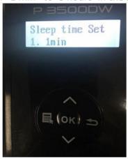
Note: When the printer is in dormant status, you can wake it up just by pressing any button or sending print task.
