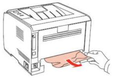
**Step4:** After clearing the jam, reload the duplex unit, check other parts of the printer, ensure that there is no jammed paper, and close the front cover, then the printer will automatically resume printing.
