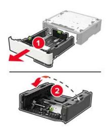
Remove the used pick roller assembly.
